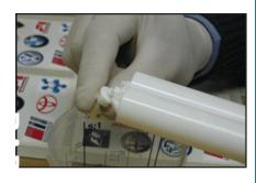
Gently break off the seal of the cartridge. Keep the seal in a safe place for resealing later.
