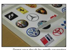
Dome your decals by gently squeezing resin onto the surface. Be careful to not apply too much or too little (this will come with practice). The resin will automatically move toward the silicon coated backing paper. Don't worry if it doesn't move all the way to the edge of the decal - you'll have time to correct this later.
