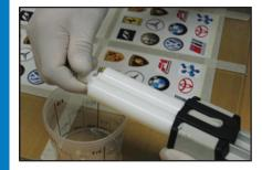
Remove the safety cap from the cartridge by turning 90° and gently pulling.
