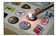
If any bubbles appear on the surface of the domed decal - use a gentle heat source (such as a hair dryer or flame) to pop the surface bubbles. Do not apply flame directly to the resin.
