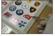
Repair decals that have uncovered areas by dragging the resin gently outwards with a scalpel or utility knife.
